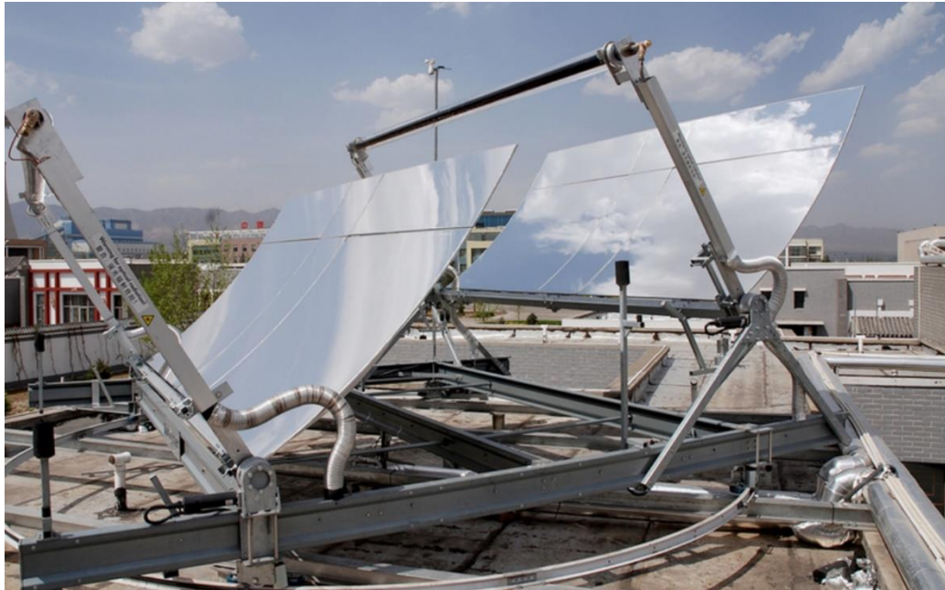
Fig. 3: Setting the reference height to the wind mast would allow for appropriate tests on the opening and closing of the SunOyster at typical day-to-day velocities.
