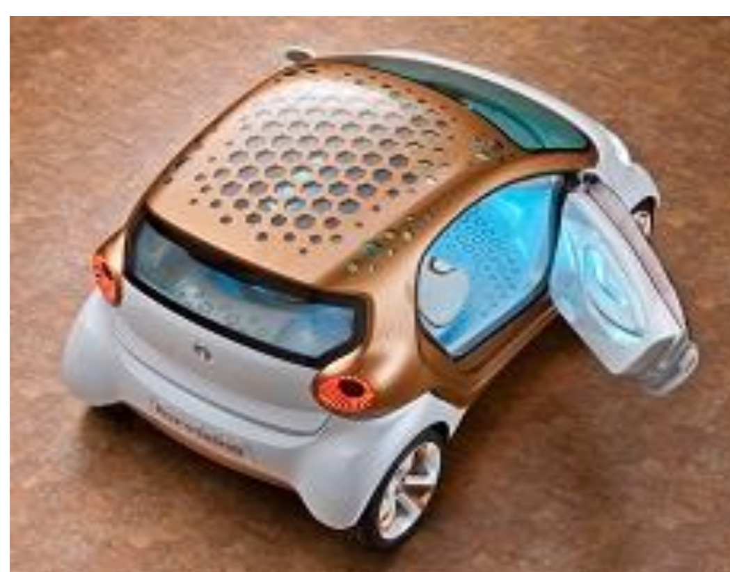
Figure 1: Car coated with spray-on OPV cells
